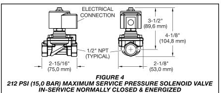
assembly may be reoriented, as necessary, by first loosening the nut on top of the coil. After repositioning the coil assembly, tighten the nut with a torque of 43 lb-in. to 53 lb-in. (4,9 N·m to 6,0 N·m).
